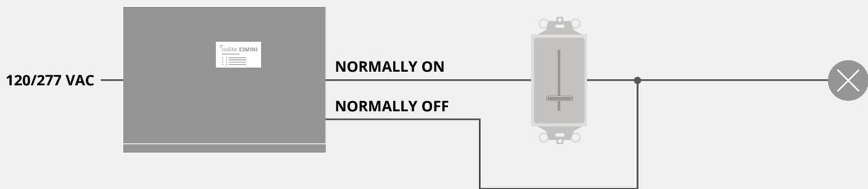
When using a traditional 2-wire dimmer, the dimmed control signal is not sent through the inverter. Instead, the inverter shunts around the phase control dimmer to short circuit the controls in an emergency. Note that while it is possible to operate the lights at a dimmed level in normal operation, when the system goes into emergency mode, the fixtures will be at 100%.
