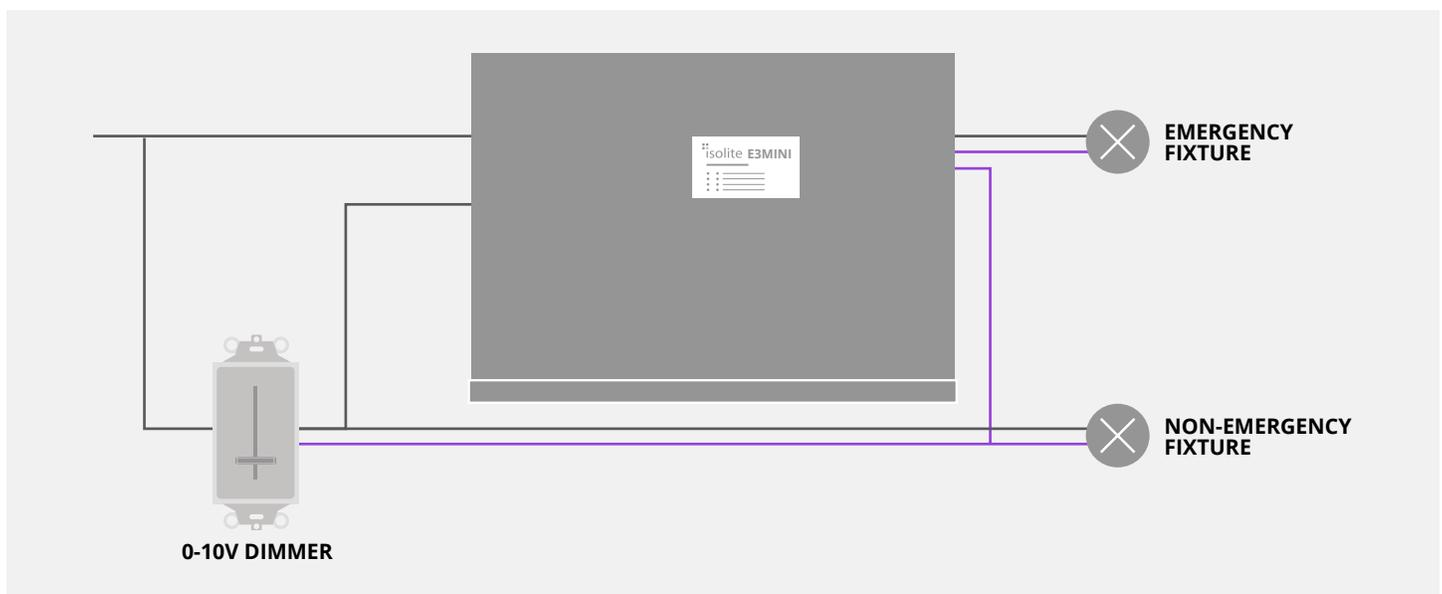
With the switched multipurpose outputs, the E3MINI allows for the integration of 3 zones of 0-10V dimming, each with **independent** control of the output dim level when in emergency mode.
