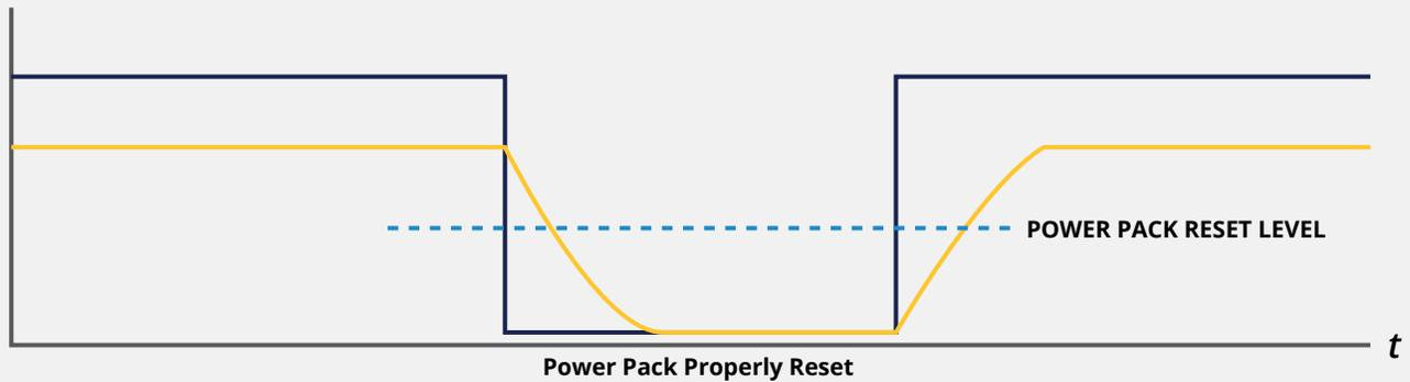
The E3MINI has a field-configurable transfer time, which defaults to a time appropriate for use with smart power packs. Faster (and slower) transfer times are selectable in the field during installation.
